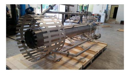
This flare tip provides a flexible method of low pressure, high volume waste gas disposal that ensures a safe and sufficient means of combustion relief flow rates from maximum emergency conditions to turn down (purge rate).
