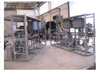
Flame front generation equipment is usually installed in a carbon steel structural frame including a sun/weather canopy.
