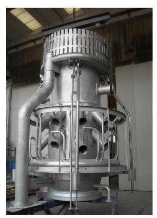
Centre steam nozzle is always required in this flare burner in order to inject steam into the centre of the flaring gas and as cooling medium for the tip internals.
