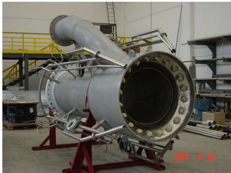
Example of Air Assisted Smokeless Flare Tip
