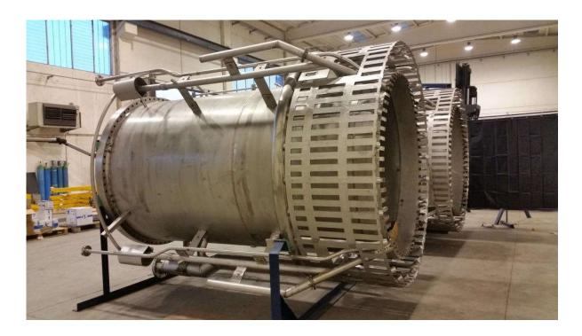
The location and orientation of these high efficiency steam nozzles ensures a very effective mixing of entrained air and flaring gases.
