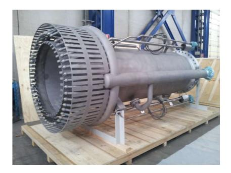
The special design of the windshield eliminates flame impingement caused by the formation of low press. zones on the downwind side of the flare.
